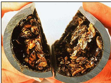
Pipe cross-section inundated with invasive Mussels
