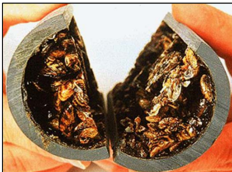
Pipe cross-section inundated with invasive Mussels
