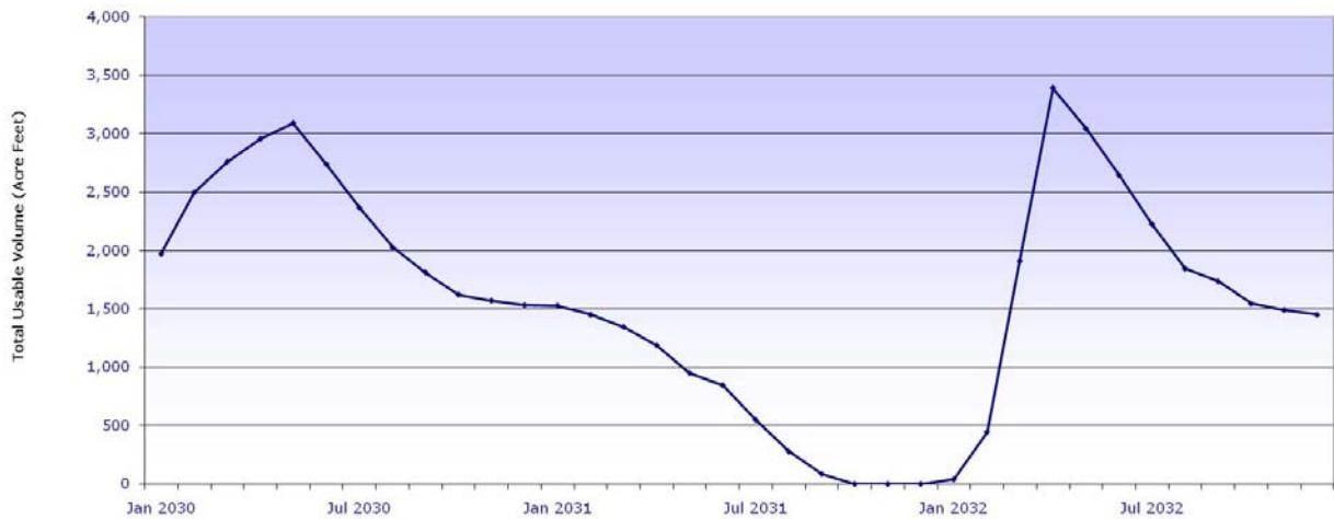
Figure 4-7. Drought Condition: Total Reservoir Storage Volumes (Medium Growth Scenario, included 2020 Compliance and 50 Percent Level of Water Conservation)
